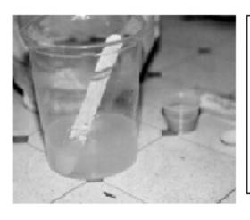
Step 5 MOST IMPORTANT. Allow the melted gelatin to cool for between 2-3 min depending on the melted temperature, until the gelatin is only warm to the touch but not gelled yet. The hotter the gelatin is when it is foamed the more it will rise and may rise out of the container.
