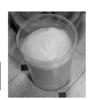
Step 7. Once it has stopped stir the foam to refine the large bubbles until an even cell structure is reached. It should be at a Meringue consistency. It is possible to reheat the foam after it has gelled. Some do this anyway and claim much better foam. They heat for about :15 to:30 sec only, in :10 sec intervals, stirring between each. By stirring you can adjust the density of the foam. This step in the procedure will require some finesse and personal judgement.
